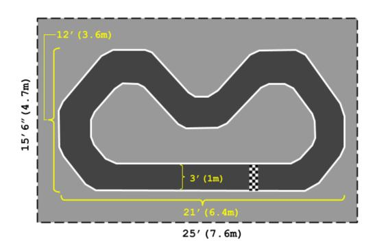
The Grand Prix circuit can be built in a similar way as illustrated. This should allow for two or three cars to race at the same time. The starting point should be located at the beginning of the straight. The track should include groups of colorful traffic cones at the end of curves for a dramatic effect when the cars leave the track and crash into them.
